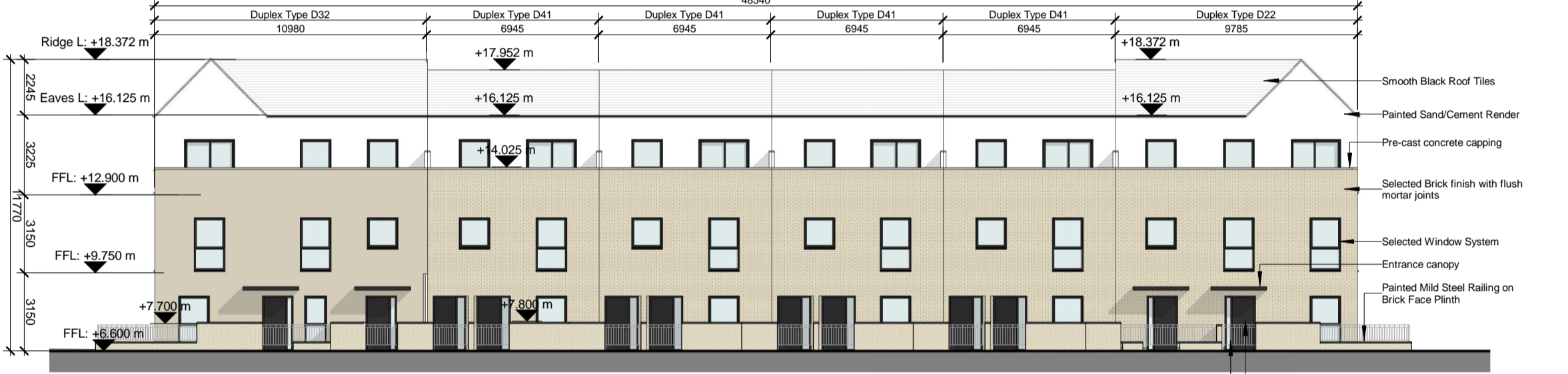
5 Duplex Block B North (Front) Elevation 1 : 200
